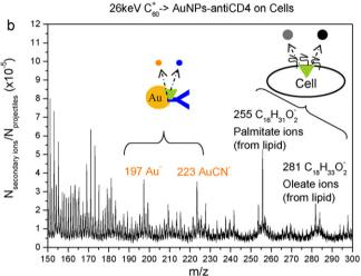
**Fig. 1.** Secondary ion mass spectrum of AuNPs-antiCD4 on Molt-3 cell micropatterned surfaces analyzed with 26 keV  $C_{60}$ <sup>+</sup> ToF-SIMS. (a) m/z 30–150 and (b) m/z 150–300
