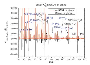
**Fig. 2.** Secondary ion mass spectra of anti-CD4 on silane glass slide (top) and silane on glass slide (bottom) impacted with  $26 \, \text{keV} \, C_{60}^+$  primary ions.
