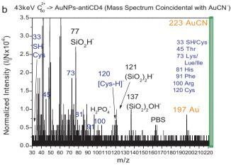
**Fig. 6.** (a) Secondary ion mass spectrum of AuNPs-antiCD4 on glass impacted with 43 keV  $C_{60}^{2+}$  primary ions and (b) coincidental ion mass spectrum of co-emitted ions with AuCN<sup>-</sup> (m/z 223) for AuNPs-antiCD4 on acrylated silane modified glass.
