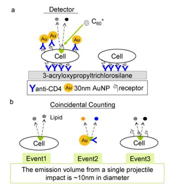
**Fig. 4.** (a) Schematic illustration of  $C_{60}^+$  impacted on a AuNPs-antiCD4 labeled cell surface and (b) individual events records.
