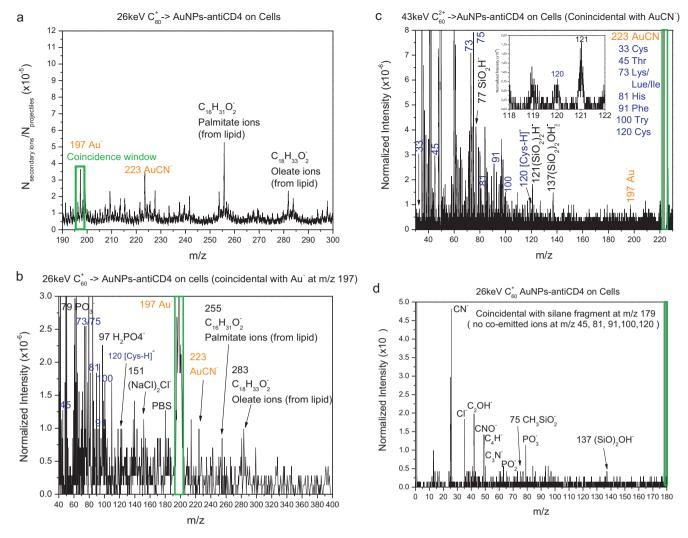
**Fig. 5.** (a) Original secondary ion mass spectrum of AuNPs-antiCD4 labeled on Molt-3 cells; (b) coincidental ion mass spectrum of co-emitted ions with Au $^-$  (m/z 197); (c) coincidental ion mass spectrum of co-emitted ions with AuCN $^-$  (m/z 223), inserted spectrum represents coincidental intensity of ion at m/z 120; (d) coincidental ion mass spectrum of co-emitted ions with silane fragment at m/z 179.
